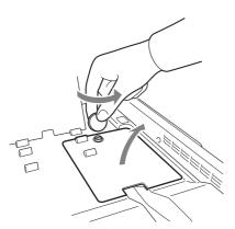
2 Insert the CompactFlash card in the expansion CompactFlash slot.
